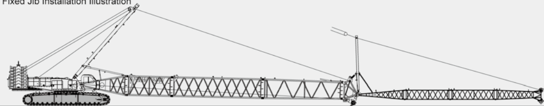
固定副臂安装示意图 Fixed Jib Installation Illustration
