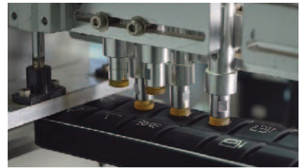
Panel Buttons: Cycled 12 Million Times
