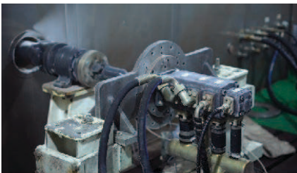
Hydraulic Pump: Low-Temperature Performance Test Under -40 °C
