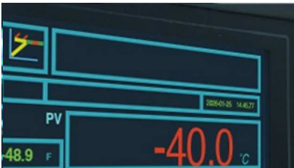
HMI Display: Low-Temperature Performance Test Under -40 °C
