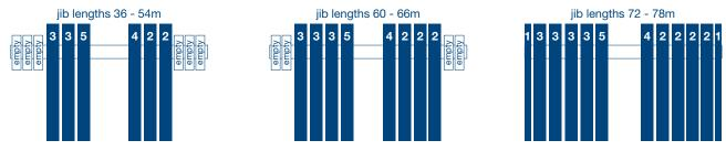
counterweight 1 = 8.7t · counterweight 2 = 13.2t · counterweight 3 = 13.2t · counterweight 4 = 14.5t · counterweight 5 = 14.5t
