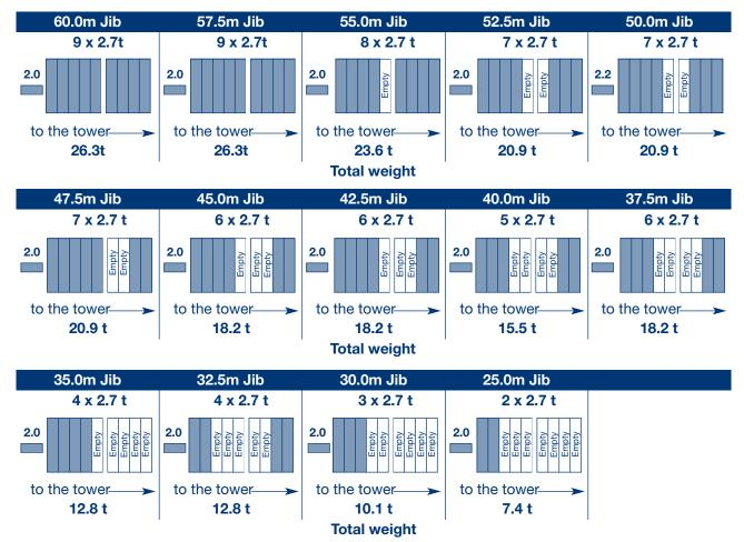
No concrete counterweights are to be fitted in the positions with a white background.
