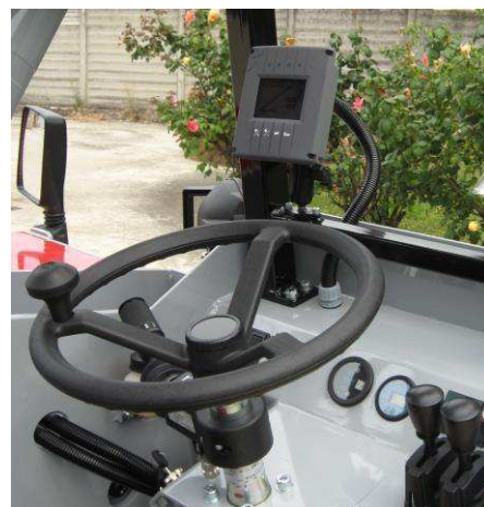
Operator's cabin with ergonomic controls and digital display for the electronic load moment indicator
