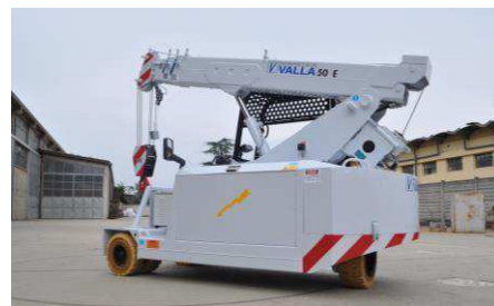
Rear steering with 180° rotation for maximum manoeuvrability
