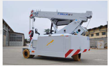
Rear steering with 180° rotation for maximum manoeuvrability
