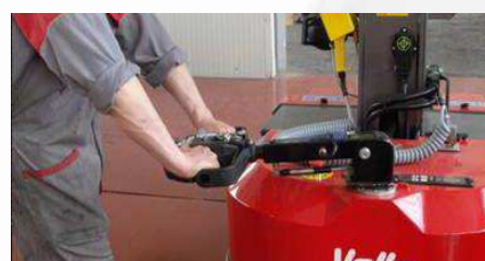
180° steering helm powered by electric motor by 180° rotation for maximum manoeuvrability
