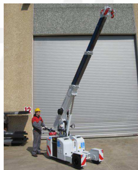
Fully hydraulic telescopic boom
