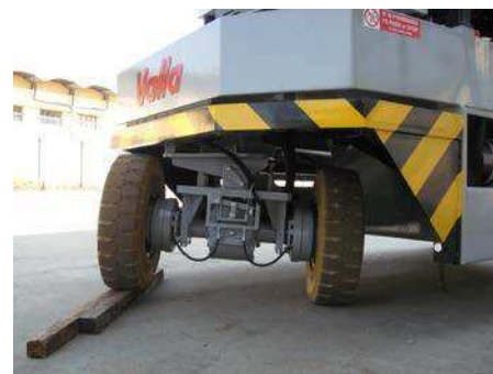
Rear steering with hydraulic cylinder between chassis and traction group for great performance also on not flat surfaces
