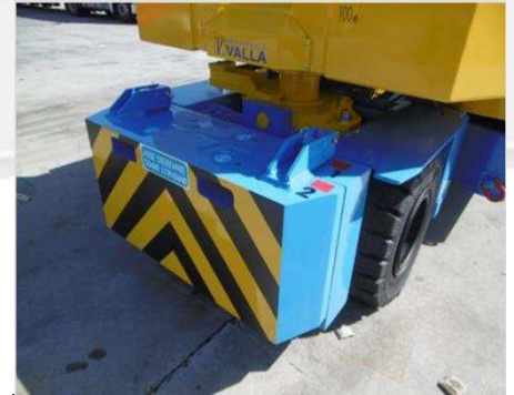
Removable ballasts to make it easier to transport the crane
