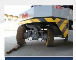
Rear steering with hydraulic cylinder between chassis and traction group for great performance also on not flat surfaces
