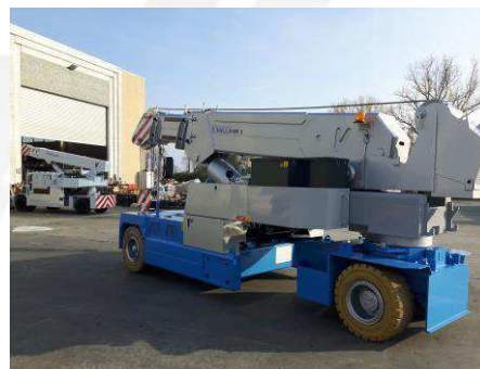
Extendable chassis to increase lifting capacity
