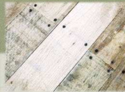
Oak Deck Trail King tilt trailers are decked with 2" nominal oak decking, not pine, and double screwed to crossmembers to prevent cupping. As a result, your deck will stand up to years of rugged service.
