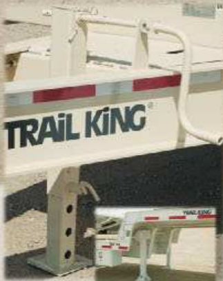
Heavy Duty Jack A 12,000-lb. heavy-duty drop-leg jack is standard equipment on all Trail King tilt models except the TKT50 tandem axle, which features telescopic pin-type parking stands.
