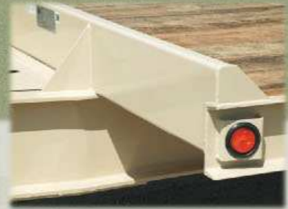
Safety Headboard The 4" safety headboard provides an extra dimension of safety and load-hauling security. And, on the TKT50 Tandem (shown here), the headboard is reinforced on the front side for even more strength.
