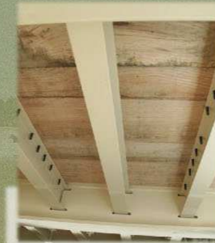
I-Beam Crossmembers Crossmembers are full-width 4" I-beams, not C-channel. And, because the mainframe and crossmembers are primed and painted with two-component polyurethane primer and paint before decking is installed, you get both strength and long-lasting durability.
