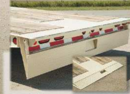
Fold-Down Approach Plate Trail King's patented tail with fold-down approach plate is designed to meet Federal under-ride protection requirements, achieve the lowest possible load angles, and provide extra protection for tail lights.
