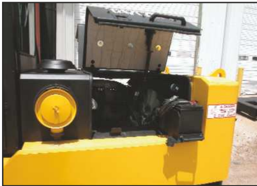
Gull-wing hood allows for easy service access to engine compartment and swing-out battery.
