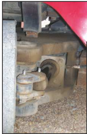
Steer cylinder is completely protected in axle housing.
