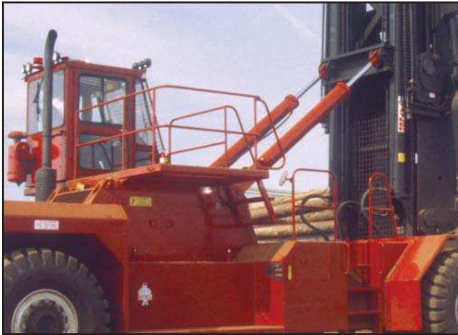
Anti-slip steps and handrails for 3 point mounting and dismounting (meets new proposed ANSI B56.1 standard)
