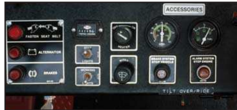
Left side operator panel
