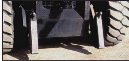
Optional log pushers to improve log stacking
