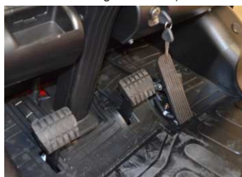
Two Pedal Hydraulic Inching & Brake and Moulded Rubber Floor Mat
