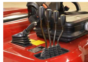
Hood Mounted Hydraulic Control Levers and Ratchet Style Hand Brake
