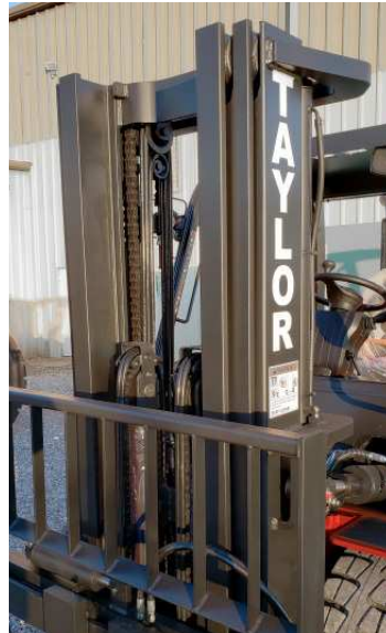
Durable Nested I-beam Design Yields Optimal Visibility
