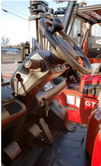
Adjustable Steering Column Pivots 30 Degrees
