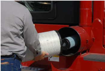
Donaldson Air Cleaner with Safety Element (Standard)
