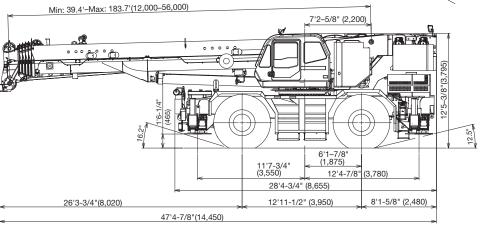
\*\*Dimension is with boom angle at -1.5 degree. () Reference dimensions in mm.
