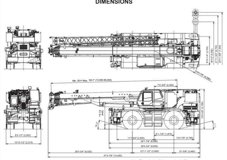
Note: Dimension is with boom angle at -1.5 degrees.
