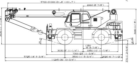
Note: Dimension is with boom angle at 0 degree.
