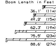
NOTE:1.Boom and jib geometry shown are for unloaded condition and machine standing level on firm supporting surface.
