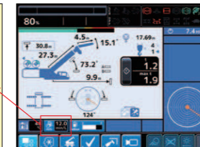
Preset menu display (during crane operation)
