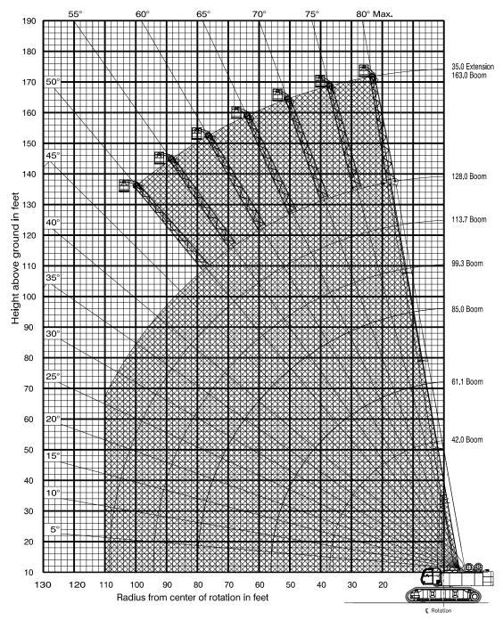
Limits of operation: Maximum load capacity = 750 lb (340 kg) Maximum radius when mounted on main boom = 110 ft (30.4 m) Minimum boom angle when mounted on 35 ft extension = 50°
