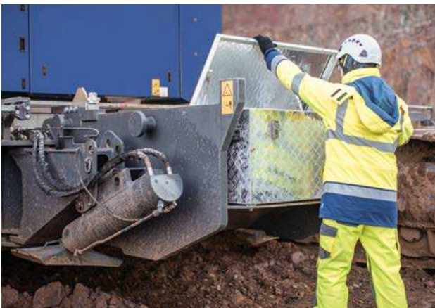
Sufficient space: the lockable aluminum box with a volume of 66 gallons is intended for tools and personal items. Chain slings are kept in another large, open box.
