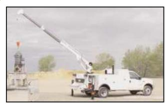
Our newest 4420 crane is the perfect service truck accessory for public utilities, municipalities, water works, and many other situations needing lifting. The 4420 features a 16,000 foot pound (2.23 ton-meters) capacity and can lift a maximum of 4,000 pounds (1,814 kg) at four feet (1.22 m). Stellar Industries is the only U.S. manufacturer in this class of crane to offer several unique features
