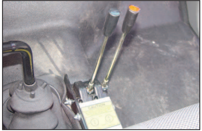
2. Engage the hook to the body by maneuvering the hooklift with the red (lift) lever and the black (tilt) lever..
