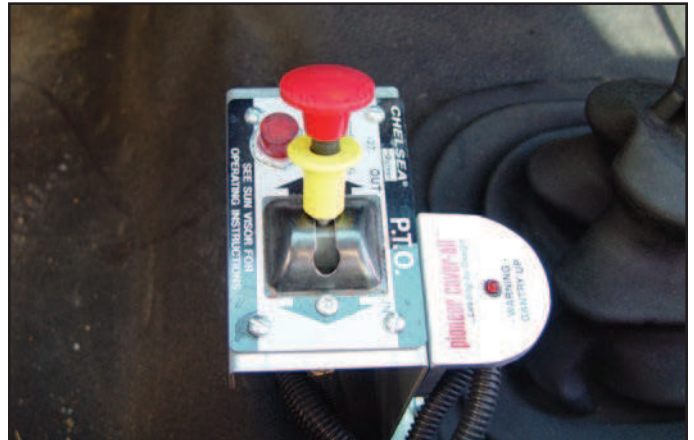
2. Put the truck in neutral and engage the PTO.
