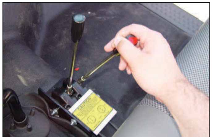
4. Pull the lift lever to dump the body.
