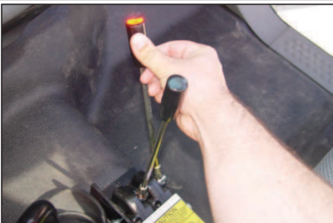
5. Wait until dumping is complete, then push the red(lift) lever until the main cylinder fully retracts.
