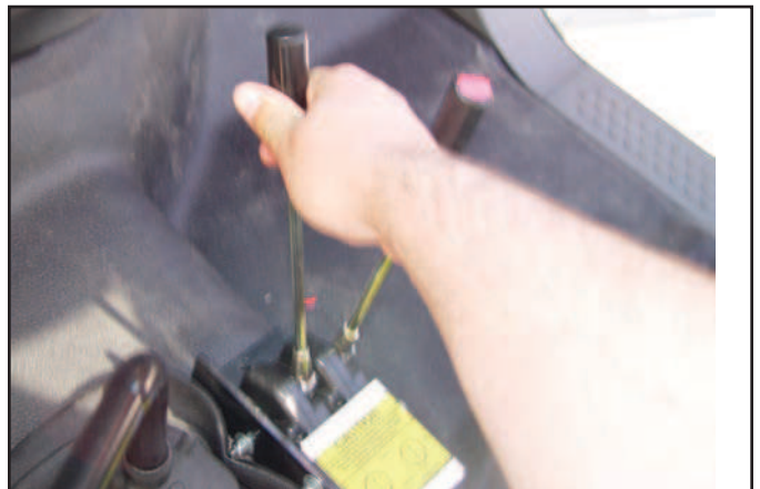
4. Push the black (tilt) lever until the tilt is fully retracted.
