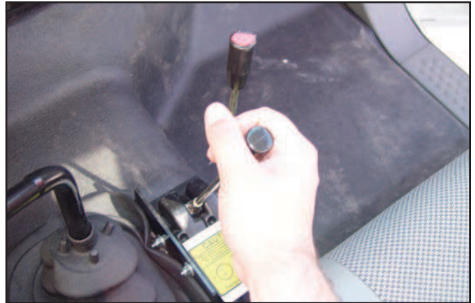
4. Pull tilt lever until full stroke is reached, thus releasing tabs.
