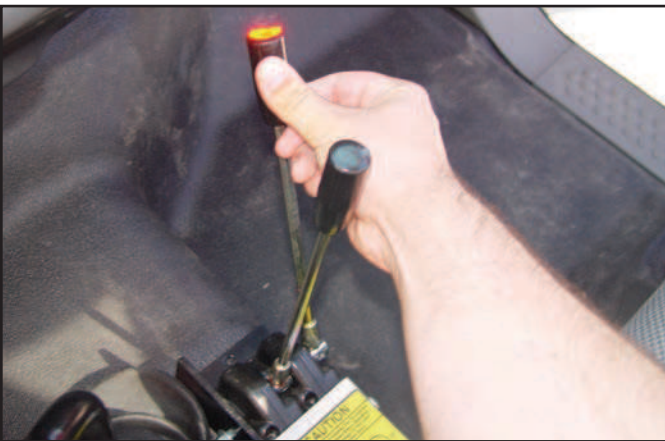
3. Push the red (lift) lever until the main cylinder is fully retracted.
