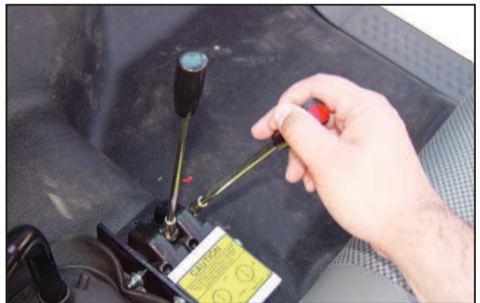
6. Pull lift lever until the body is on the ground and can be detached. Return the hooklift to the stored position and disengage the PTO.
