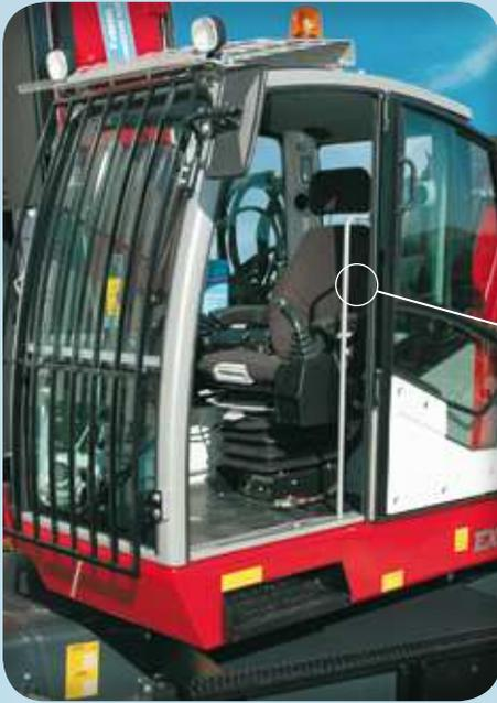
**Operators cabin** with large windows for a better visibility. The front window, with double wiper, opens, completely disappearing under the top of the cab.
