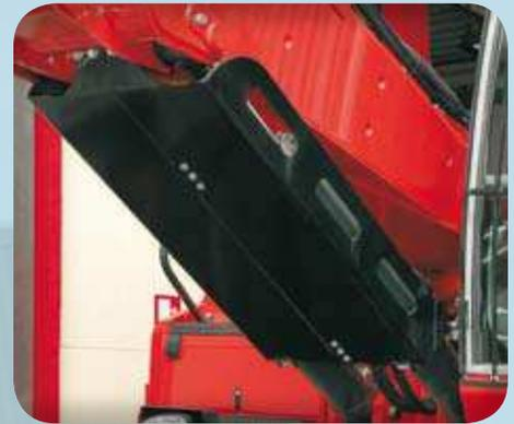
**Hoist cylinder's rods protection** available on request.
