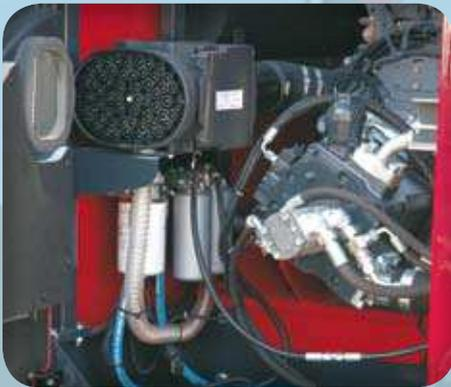
**Air cleaner** with self-cleaning micro-cyclones vacuum system standard included: lower maintenance time and costs, higher efficiency for the air filter, optimum working conditions for the diesel engine.
