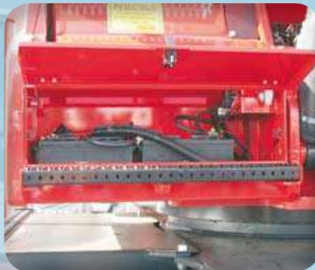
**Lockable battery box** with general on/off switch standard included
