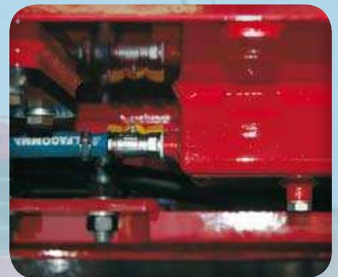
**Safety taps** on the diesel and oil tank for a quicker and easier maintenance of the machine
