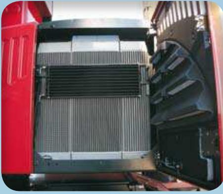
**Large radiators**, in aluminium with large-meshes to allow a better thermic exchange avoiding occlusion of air passages. A thermostatic reversible fan with new aerodynamics profiles of the blades is as standard included: less noise, less diesel consumption, radiator always clean, less heating time in wintertime, quicker heating into the cabin in wintertime.
