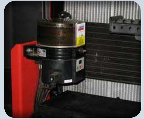
Centralized automatic greasing system (as option), to make easier service operations.
