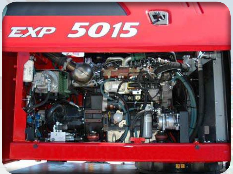
The large bonnet , ensures an extremely easy and safe access to all maintenance points.
