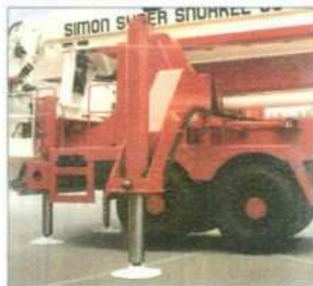
Four jacks and stabilisers
