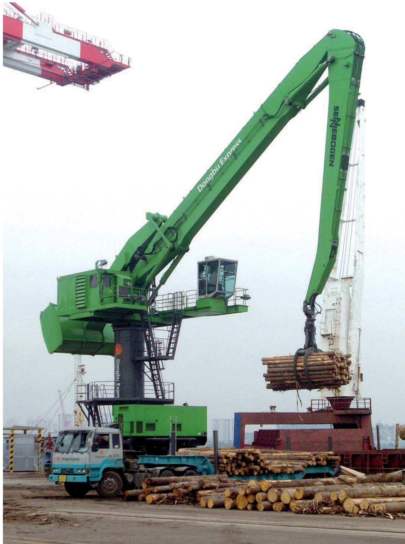
880 EQ - Pylon 7 m - Ausrüstung K33 | 880 EQ - pylon 7 m - equipment K33
