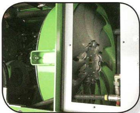
Hydraulic driven fan with flow optimized fan blades, reversible to keep the coolers free of debris.
