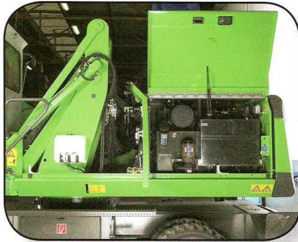
Access from the ground to hydraulic components, air filter, diesel tank, central lubrication, electric panel and battery disconnect switch.
