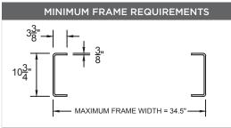
Minimum section modulus per rail = 17.8 in.<sup>3</sup> Minimum yield strength = 110 KSI
