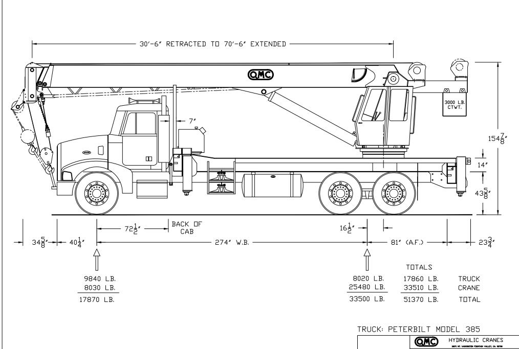
ALSO SHOWN ARE OPTIONAL EQUIPMENT WHICH INCLUDE FLY AND AUXILARY REEVING PACKAGE.
