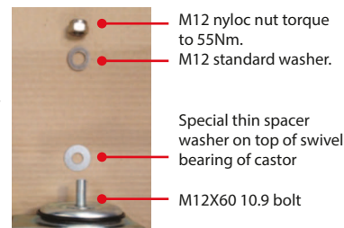
Castor mounting bolt Swivel bearing head should feel free to rotate and not loose
