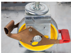
Foot pedal distortion as a result of a significant impact; it is likely the top plate and bearing will be distorted as well.
