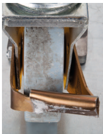
Foot pedal distortion as a result of a significant impact; it is likely the top plate and bearing will be distorted as well.
