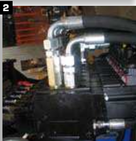
2 DISTRIBUTORE IDRAULICO PROPORZIONALE COMPENSATO PVG 32 CONTROL VALVE BLOCK COMPENSATED DISTRIBUTEUR HYDRAULIQUE PROPORTIONNEL COMPENSÉ HYDRAULISCHER PROPORTIONALER KOMPENSIRTER STEUERBLOCK DISTRIBUIDOR HIDRAULICO PROPORCIONAL COMPENSADO PVG 32
