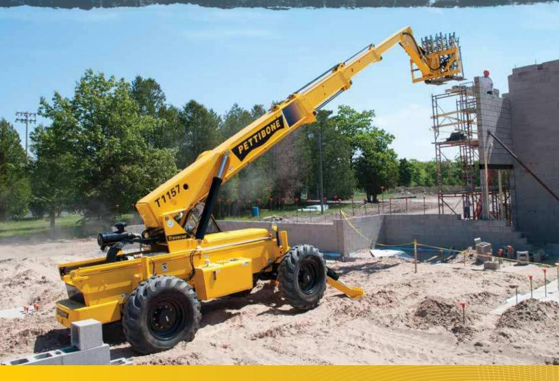
The Traverse<sup>™</sup> T1157 from Pettibone<sup>®</sup> is ruggedly built and engineered to deliver results for the long haul. High lift capacity and reach, along with 70 inches of horizontal boom transfer, makes easy work of landing loads. The T1157 also offers exceptional operator visibility and superior maneuverability for enhanced efficiency. Responsive hydraulics ensure smooth operation for any job application.
