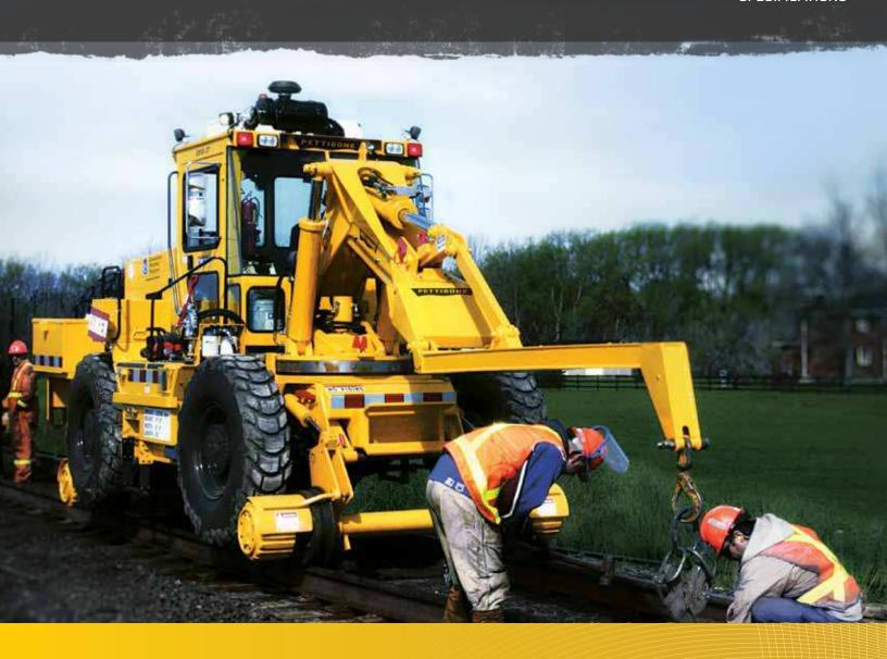
Designed to tackle a variety of rail applications, the Pettibone® Speed Swing™ 445E is a versatile machine that provides the power to lay rails, set ties or clear the path ahead. The unit features a turbo diesel engine and 180-degree boom rotation for enhanced productivity. Offering precise hydraulics, numerous attachments and the ability to work both on and off the rails, the Speed Swing 445E is equipped for any rail task.
