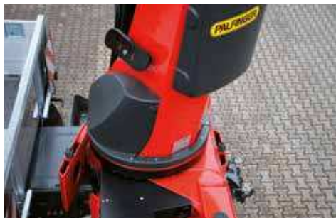
CONTINUOUS SLEWING SYSTEM UNRESTRICTED MOVEMENT
