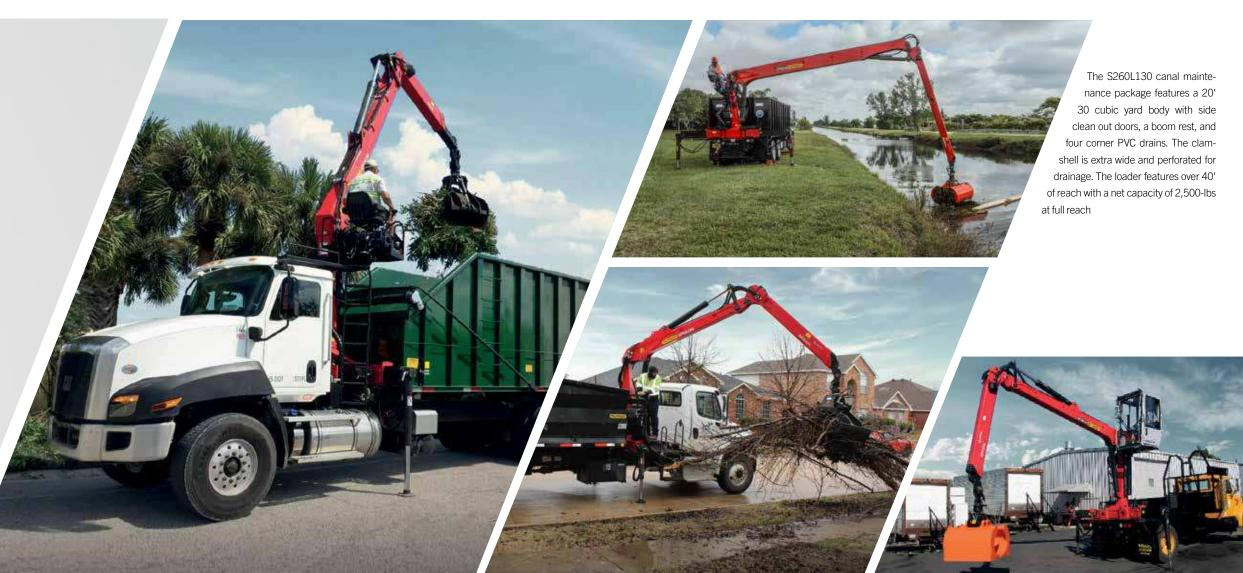
The M110L80 & Q150L80 packages are designed for single or tandem axle trucks. These loaders provide options for longer reaches (32') with higher capacities (3,970-lbs @ 25') and numerous control variations. The out and down stabilizers provide increased stability for those heavy picks.
