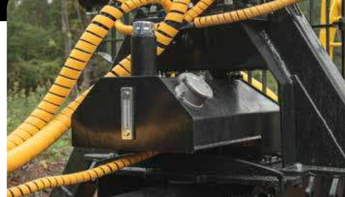
Different oil tanks for independent hydraulic system from tractor
