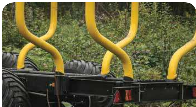
Frame extension to maximize the loading length.
