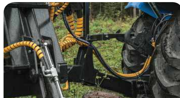
Straight and angle draw bars with different fastening options for draw bar loop.
