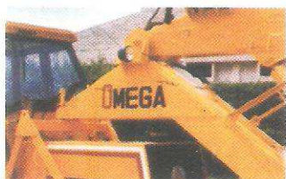
Re-enforced robust Goose neck for heavy duty application.
