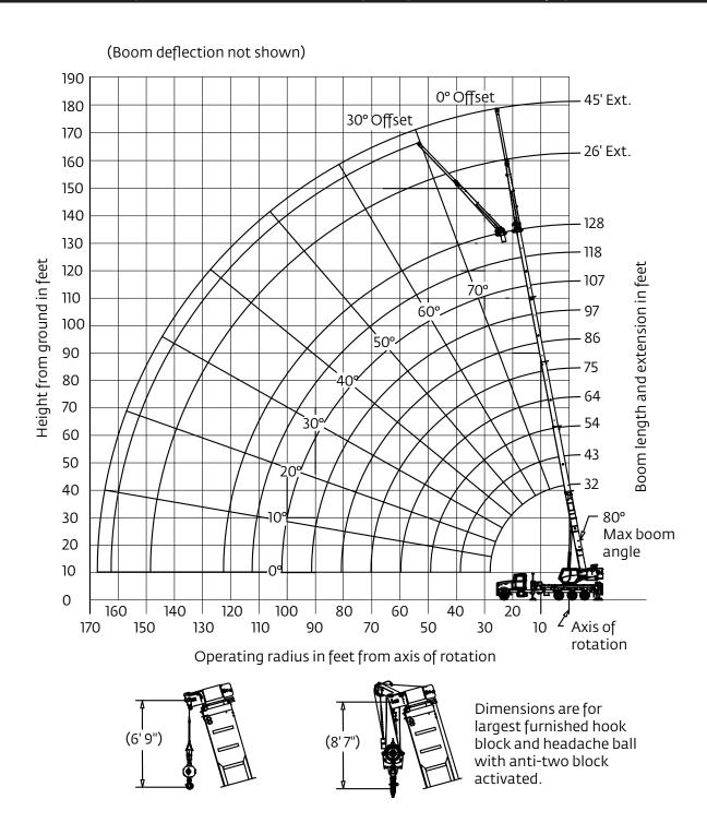
\*This drawing shows the physical reach of the machine. Always refer to the load chart to see which portions of this diagram are valid for the specific machine configuration and where the loads are structurally or stability limited.
