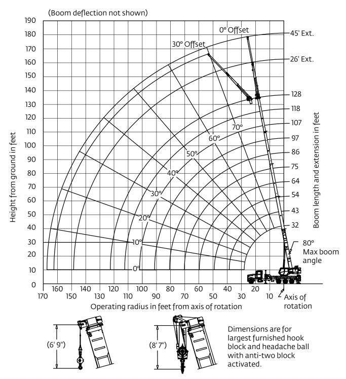
\*This drawing shows the physical reach of the machine. Always refer to the load chart to see which portions of this diagram are valid for the specific machine configuration and where the loads are structurally or stability limited.
