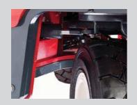
> Rear flat race steer bearing for longevity and ease of maintenance
