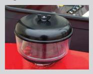
> The air filter pre-cleaner helps keeping feathers and dust out of the air filter The operator compartment is fully enclosed with toughened glass panels for winter use and can be easily removed for open air use during warm weather months.
