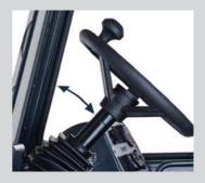
> Tilt adjustable steering for optimum operator interface
