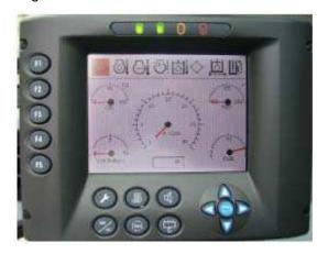
Once the engine data has been reviewed by the operator, press and release the page pushbutton to check the level of the machine. Press and release the page pushbutton again to set up the RCI.
