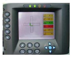
The display will change to the last selected program and part of line in a shut off condition (Red Stop Symbol and Red Light). If the selected program is correct, confirm by pressing and releasing the **ENTER pushbutton.** The system will reset in a normal operational condition.
