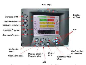
Press and release the pushbuttons to select the functions or change the function. System Selection of Program, Parts of Line, Engine RPM settings, and confirmation is on page 25.
