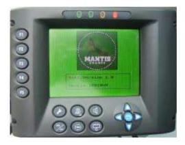
The display will briefly indicate the RCI screen and then go directly to the engine screen for engine data.
