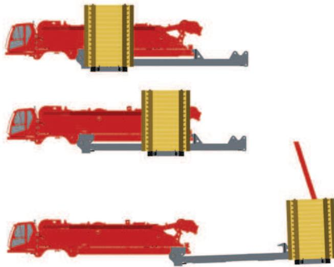
In VPC-MAX configuration, the counterweight tray moves to the end of the VPC-MAX beam prior to beam extension, thus minimizing tailswing and increasing job site mobility.
