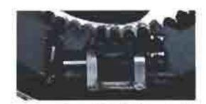
SWING LOCK: Air-controlled, spring-loaded gear segment engages swing gear for positive locking
