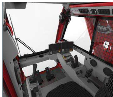
New Wide Cab with Crane Control System (CCS)
