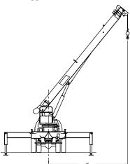
2. Loaded boom angle ( $\angle$ ), as shown in the load chart columns headed by  $\angle$ , is the included angle between the horizontal and longitudinal axes of the boom base after lifting rated load at rated radius (see below).
