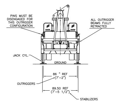
USE THIS CHART ONLY WHEN OUTRIGGERS AND STABILIZERS ARE FULLY RETRACTED
