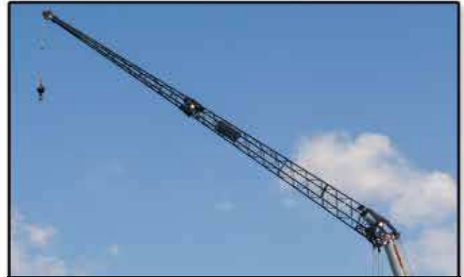
38-64 ft (11.67-19.5 m) two-piece bi-fold, lattice attachment with 2°, 15°, 30°, and 45° offsets.
